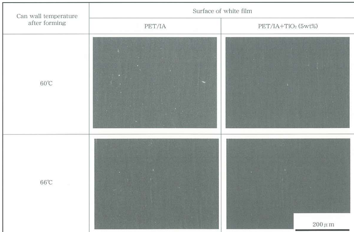
Fig.7 SEM images of the can wall after forming (C350TULC, 7mm from the upper side of can)
