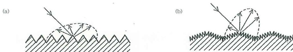
Fig.7 Model of light reflecting surface
