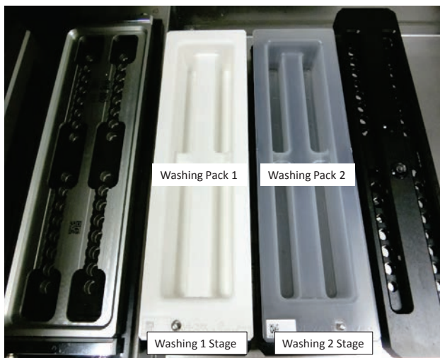
Fig.5 Washing stage of BIOSHOT HT-32 for washing GENE SILICON after hybridization.
