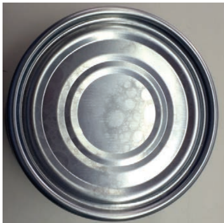
Fig.1 Retort blushing of the DRD can.
