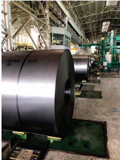
Fig.8 Appearance of cold rolled coil at delivery walking beam conveyor.
