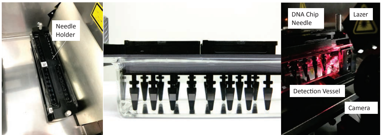
Fig.6 Detecting stage of BIOSHOT HT-32 for detect fluorescence.
